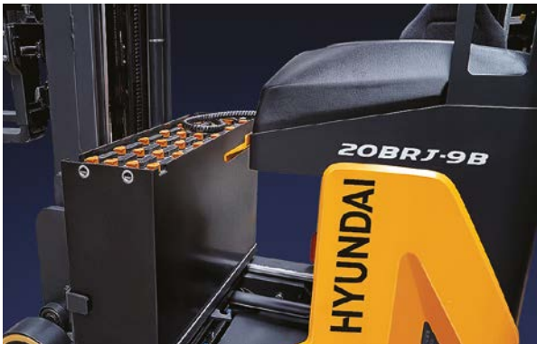
Side battery extraction.
