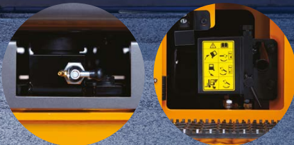
Cabin Tilting Switch
